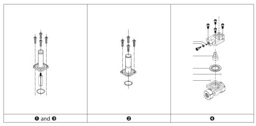
To get a complete acatuator and diaphragm service 1), 2) or 3) and 4) should be ordered. Fx. For EV220BW 15 / G1/2 NC needed ordering are 132U8080 and 132U8016.
